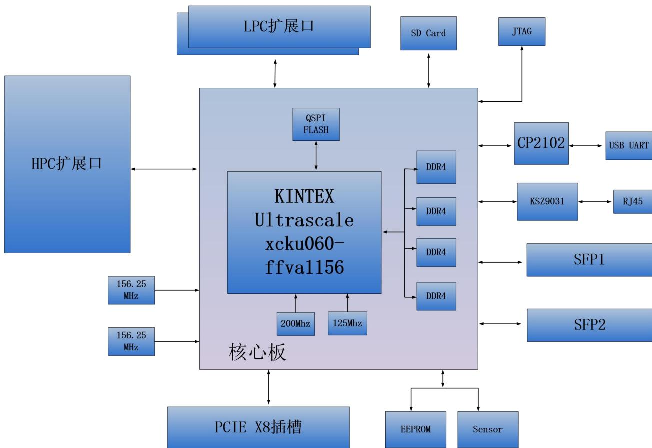
Through this diagram, you can see the interfaces and functions that the AXKU062 FPGA Development Board contains:
