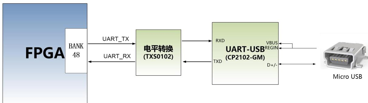
Figure 2-5-1 USB to serial port schematic diagram
