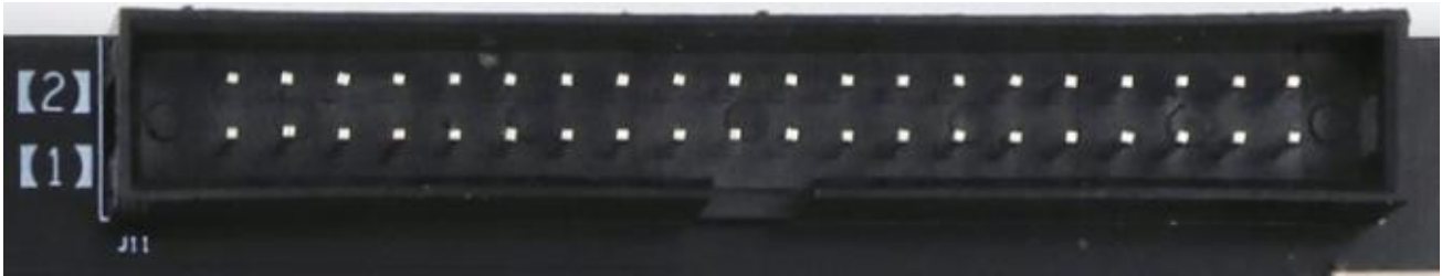
Figure 3-11-2: Expansion header J11 on the Carrier Board
