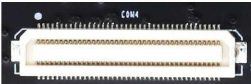
Figure 2-9-4: Board to Board Connectors CON4 on the Core Board
