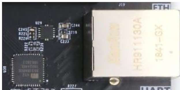
Figure 3-3-2: Gigabit Ethernet interface on the Carrier board
