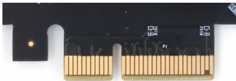
Figure 3-4-2: PCIe x2 on the Carrier Board
