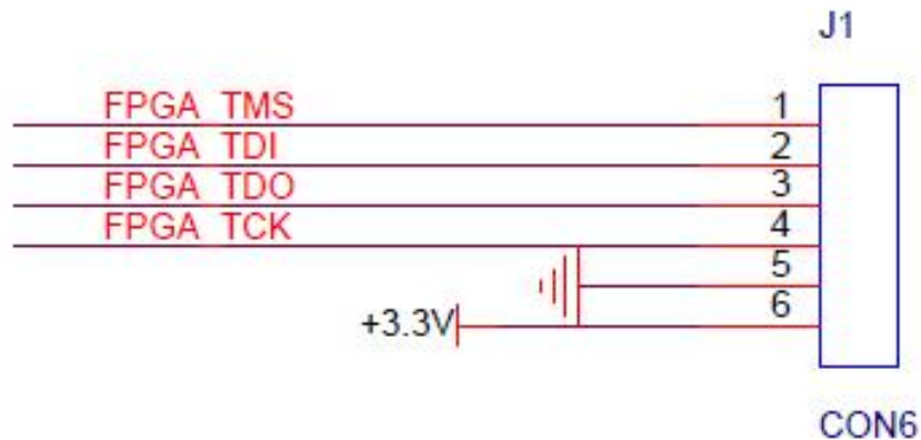
JTAG Interface Schematic
