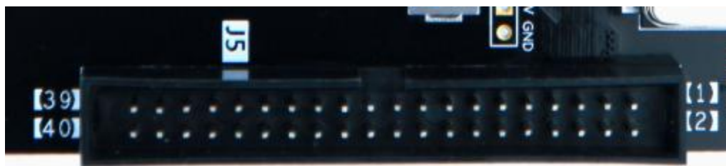
Figure 3-11-4: Expansion header J5 on the Carrier Board
