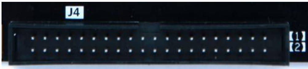
Figure 3-11-2: Expansion header J4 on the Carrier Board
