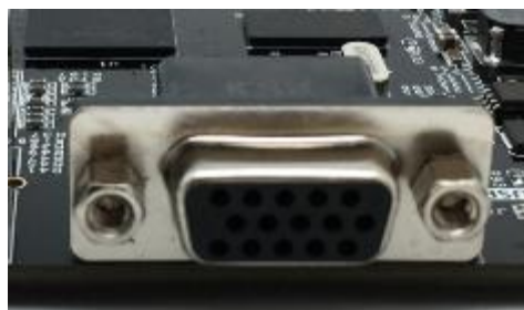
Figure 3-4-3: VGA Display Interface on the Carrier Board
