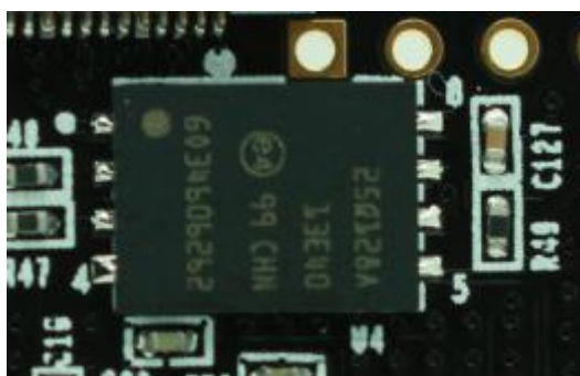
Figure 2-5-2: QSPI on the Core Board
