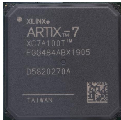
Figure 2-2-2: FPGA chip on board
