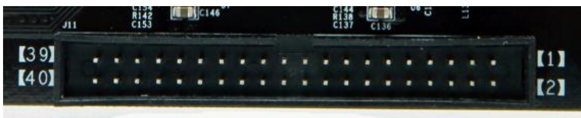
Figure 3-6-2: Expansion header J11 on the Carrier Board
