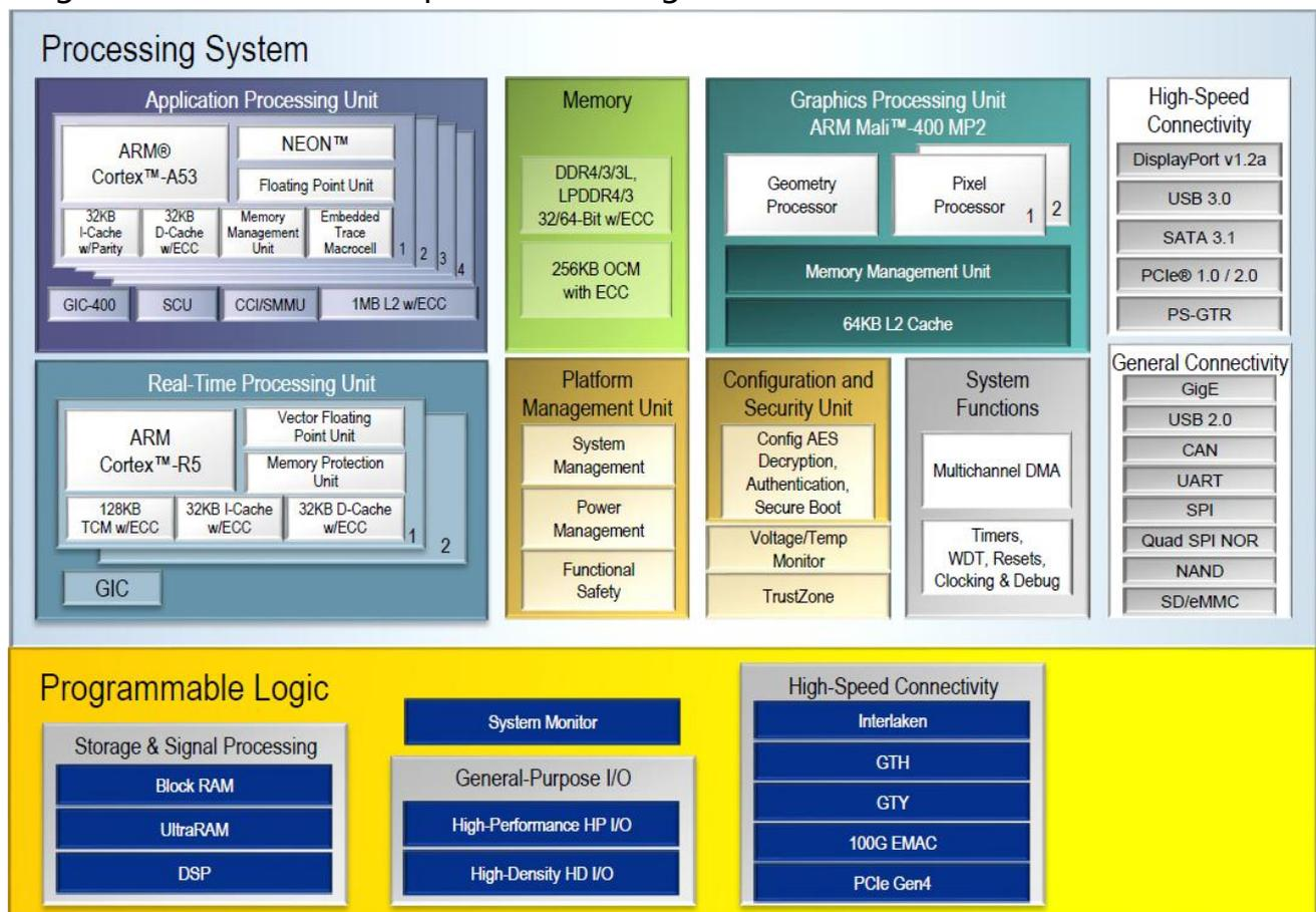
Figure 2-2-1 Overall Block Diagram of ZYNQ ZU19EG chip
