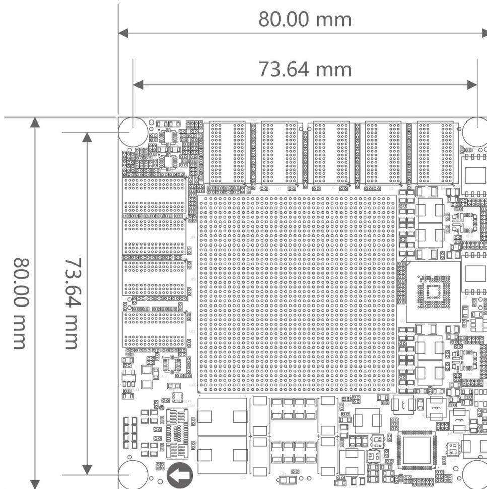
Figure 2-8-1: ACU19EG Core Board Form Factors (Top View)
