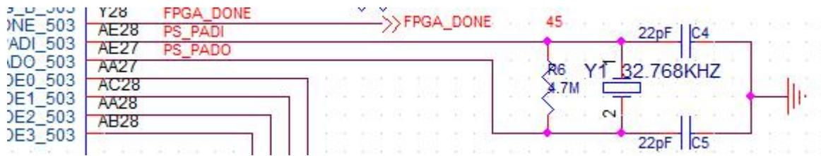
Figure 2-6-2: Crystal Oscillator for RTC
