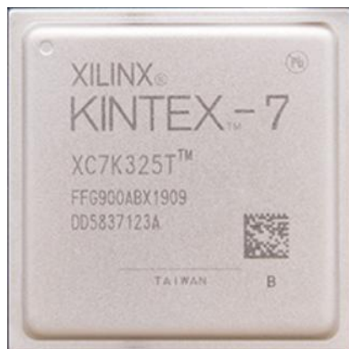
Figure 2-2: FPGA chip on board
