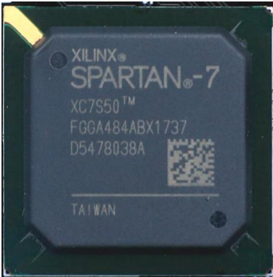
Figure 2-2-2: FPGA chip on board
